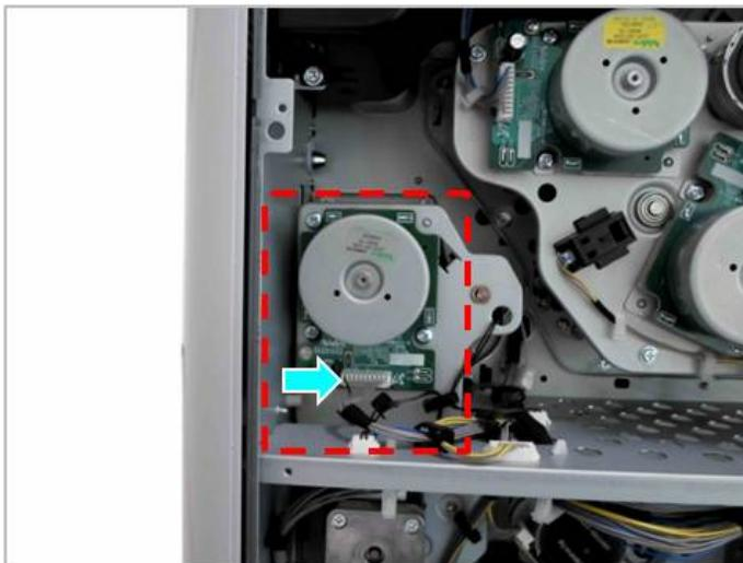
5. If the connection is OK, turn the machine on. Enter SVC mode. Select motor test: Diagnostics > Engine Diagnostics > Engine Test Routines > 100-0000
